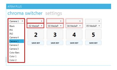
C. <u>Click on a number to perform</u> a cut in the PGM. As a PGM is automatically selected MEDIA1 and set the FILL, BACKGROUND and Chroma key's settings. Now use the handles on the right side of the application to <u>set the key parameters</u>. Fine setting of parameter can be done using the mouse wheel over the parameter slider. After that <u>click SAVE KEY</u> which will assign current key setting to desired Chroma switch. Key setting is not assigned and saved automatically.
